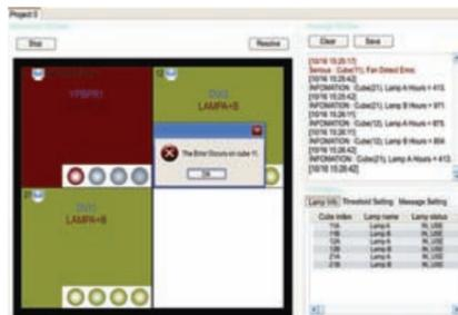
Each cube is fully IP addressable with multiple levels of alarm. This provides the operator with direct feedback on the status of the system. Whether it's the number of hours of a lamp or a defective fan, chassis intrusion or increased temperature of the CPU, the operator will be automatically notified via the pre-defined alarms on his screen.
